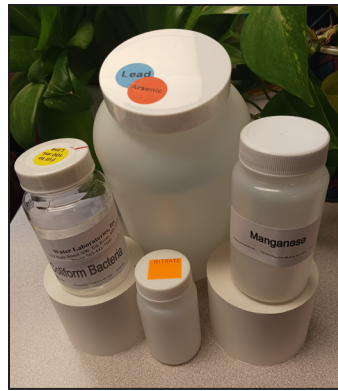
Kits test for bacteria, nitrates, arsenic, lead and manganese. Photo Courtesy of Mille Lacs SWCD
