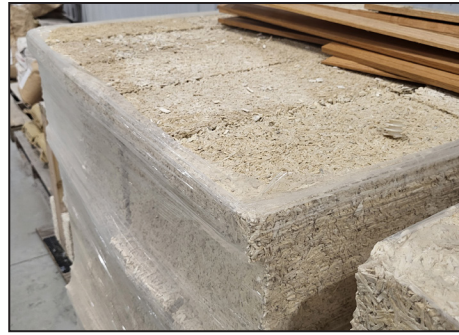
Hempcrete blocks ( center ) are made by mixing hemp ( left ), a lime-based binder and water. Photo Credits: Ashley Rezachek, BWSR Right: Danny Desjarlais, hempcrete construction project manager, stands in front of a prefabricated hempcrete wall panel at the Lower Sioux Indian Community's hemp manufacturing facility. Photo Credit: Denise Lauerman, BWSR
