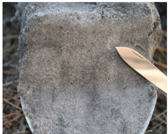
Figure 25.—Indicator S6, Stripped Matrix. This indicator requires diffuse splotchy patterns with rounded areas stripped of organic matter or iron as exemplified in this photo of a horizontal cross-section of a profile.
