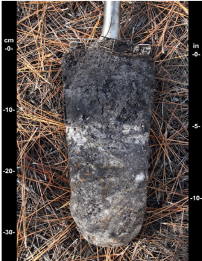
Figure 27.—Indicator S8, Polyvalue Below Surface. The diffuse splotchy pattern of black (value of 3 or less and chroma of 1 or less) and gray (value of 4 or more and chroma of 1 or less) below a black surface horizon is evidence of organic matter that has been mobilized and translocated. This soil also meets the requirements of indicator S5, Sandy Redox.
