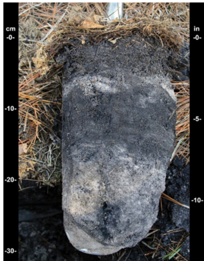
Figure 28.—Indicator S9, Thin Dark Surface. A dark surface horizon about 5 cm thick overlies a thin layer with value of 4 or less and chroma of 1 or less. Directly below the second layer is a spodic horizon, starting at a depth of about 7 cm.
