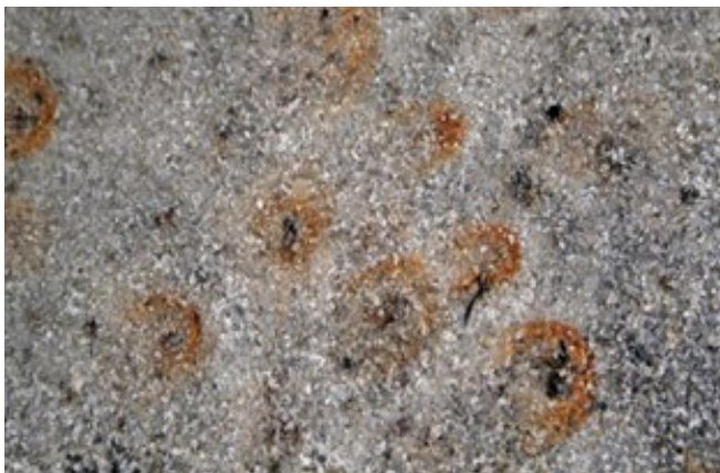
Figure 24.—Indicator S5, Sandy Redox. A close-up of the layer in figure 23 that has chroma of 2 or less and at least 2 percent redox concentrations.
