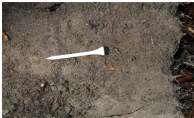
Figure 33.—Indicators F6, Redox Dark Surface and F7, Depleted Dark Surface. An example of both depletions and concentrations in a dark matrix.
