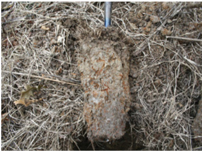
Figure 46.—A depleted matrix with value of 4 or more and chroma of 2 or less. Redox concentrations occur as soft masses and pore linings.
