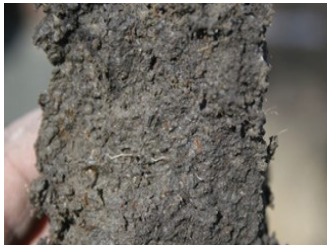
Figure 31.—Indicator F6, Redox Dark Surface. A soil that meets the requirements of indicator F6 must have a dark surface layer with value of 3 or less and chroma of 2 or less and redox concentrations in the dark layer.
