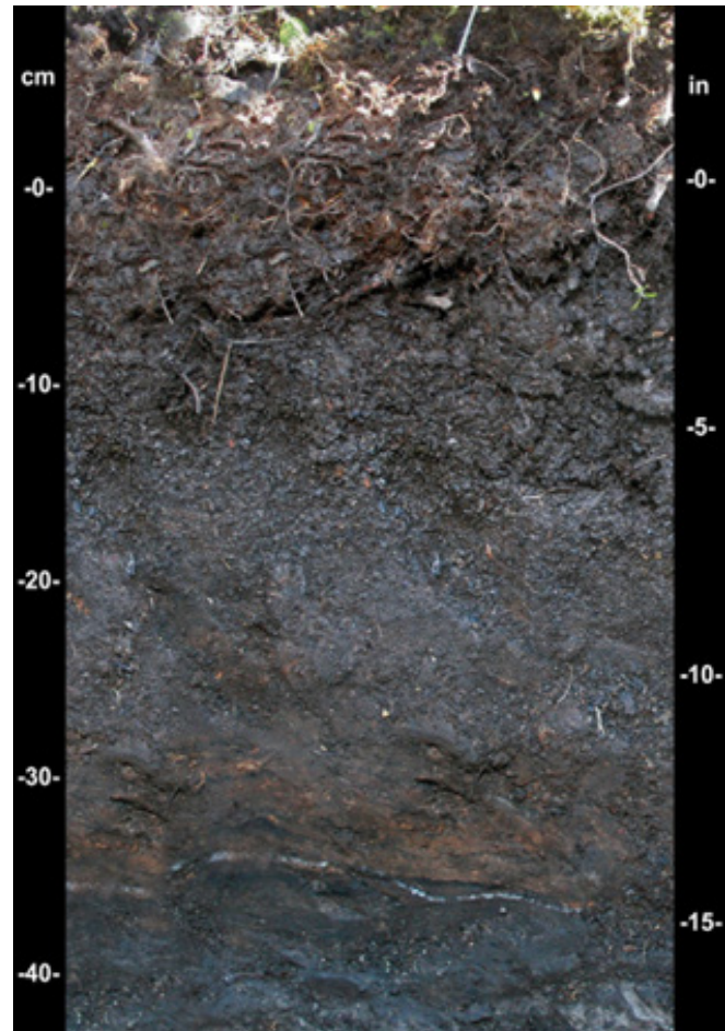
Figure 9.—Indicators A2, Histic Epipedon and A3, Black Histic. This soil meets the depth criterion of A2 and the color and depth criteria of A3. The black color, a requirement of A3, results from the accumulation of organic matter when the soil is saturated and anaerobic.
