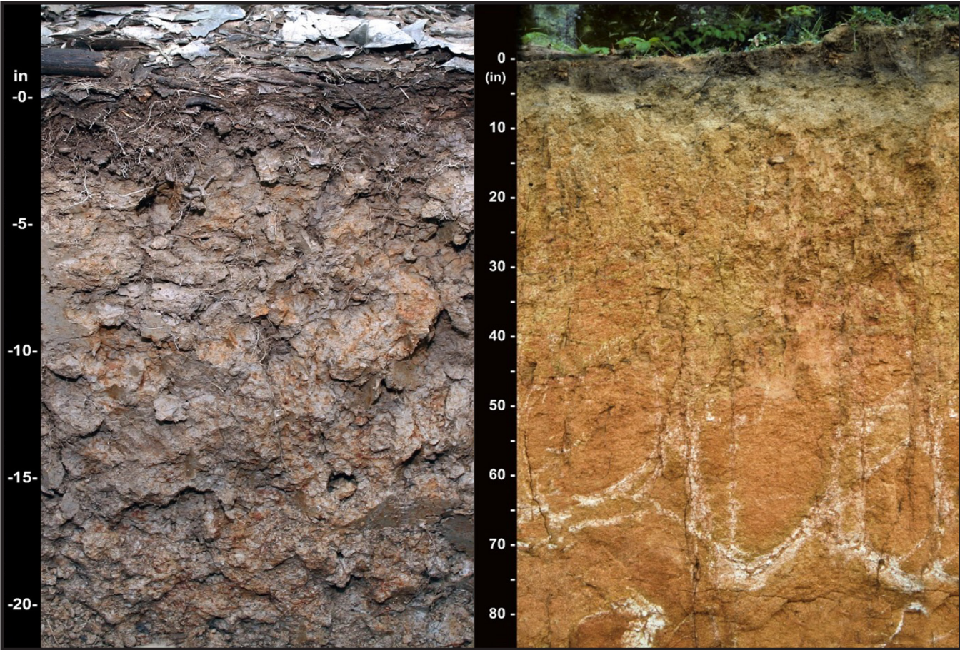
Figure 1.—The soil on the left is a hydric soil. It meets the requirements of indicator F3, Depleted Matrix. The soil on the right has indicators of wetness (redox depletions) too deep in the soil profile to meet the requirements of any field indicator and does not meet the definition of a hydric soil.
