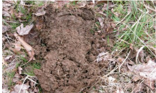
Figure 34.—Indicator F8, Redox Depressions. F8 requires only 5 percent redox concentrations in the upper part of the soil and has no matrix color requirement.
