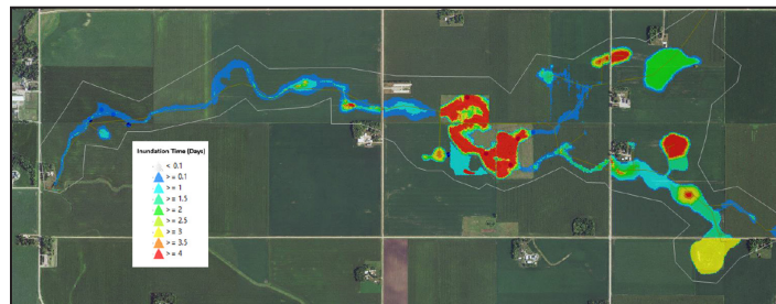
The Infoworks ICM model is used to evaluate the inundation time of a proposed storage area along a ditch system in Faribault County. This is compared against existing conditions and shown to producers to illustrate how flood levels could change if they decided to add storage to their property. Image Courtesy of ISG Inc.
