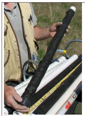
**Figure A6:** Well screen wrapped in geotextile fabric.
