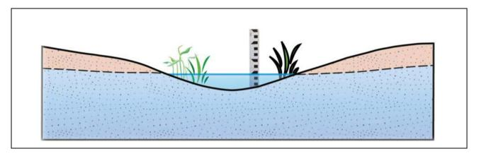
**Figure 9:** Surface water levels can be useful for estimating water table position in adjacent areas or for establishing a regional base level.
