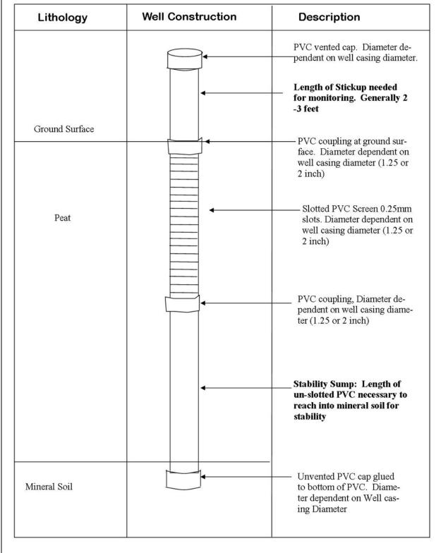
Figure B1: Shallow Peat Water Table Well Installation
