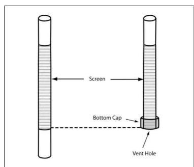
**Figure A3**: Modifying commercial well screen for wetland hydrologic monitoring. (U.S. Army Corps of Engineers, 2005).
