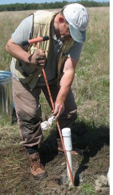
Figure A10: Adding (left) and tamping (right) bentonite.
