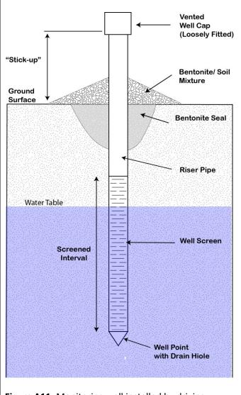
Figure A11: Monitoring well installed by driving.
