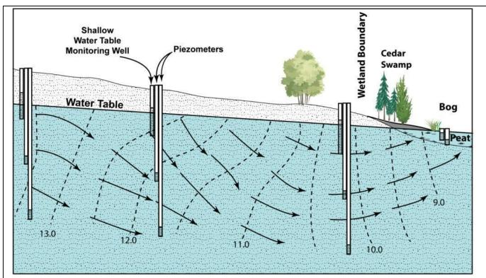
**Figure 18:** An example transect of shallow monitoring well/ piezometer "nests" as might be installed to investigate ground water flow at a wetland margin. The water levels measured in the piezometers give the hydrostatic pressure or "head" at specific depths. These can be used to construct a "flow net". Contouring the head data yields lines of equal head ("equipotential" lines – dashed lines in figure), from which localized flow directions can be determined (arrows).
