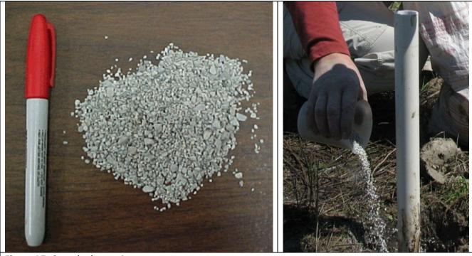
Figure A7: Granular bentonite.
