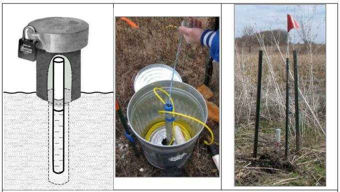
**Figure A5** Left: steel protective casing and locking cap. Center: Improvised protective housing for water level data logger. Right: Protection posts.
