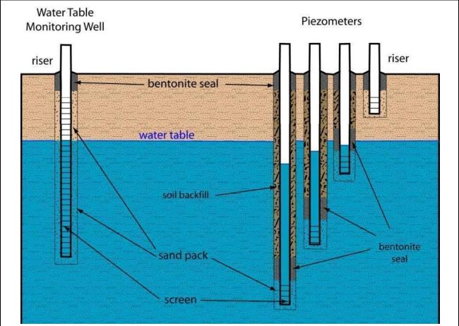
**Figure 14:** Water table well and piezometers. Note that the water levels measured in the piezometers are not necessarily the same as the water table. (Here the water levels in the piezometers indicate a downward component to ground water flow.)
