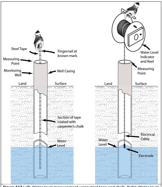
**Figure A12** Left: Water level measurement using steel tape and chalk. Right: Water level measurement using electric water level meter.
