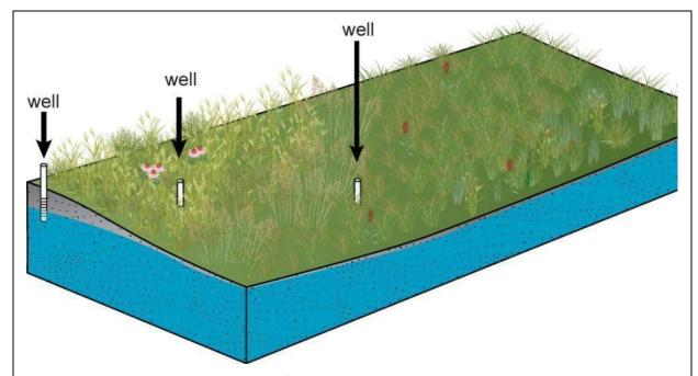
Figure 16: Monitoring using a transect of shallow wells.
