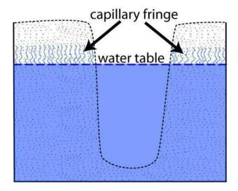
Figure 7: Water table and capillary fringe.
