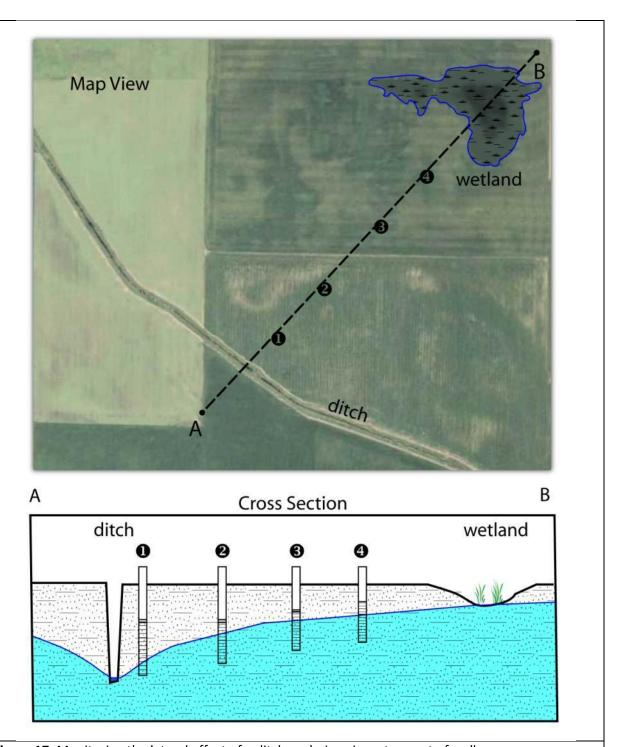
Figure 17: Monitoring the lateral effect of a ditch or drain using a transect of wells
