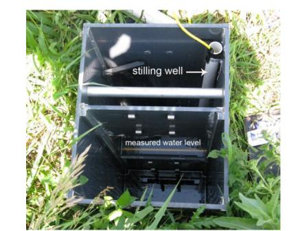
Figure 11: Water control structure with stilling well and data logger.
