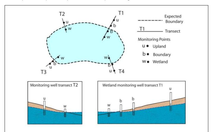
**Figure 19:** Example of monitoring well transects perpendicular to wetland boundary designed to confirm wetland boundary based on ground water level measurements.
