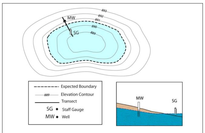
**Figure 20:** Example of how using professional judgment informed by topographic survey data and soils information, can make for a smaller, more efficient, but equally effective monitoring installation.
