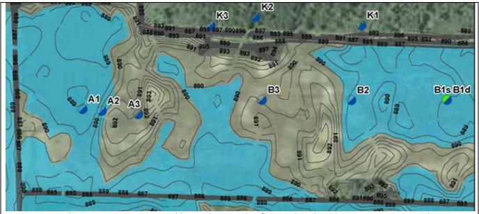
Figure D4: Map showing area where water table is within 12 inches for ≥ 14 days during a growing season. Based on water level elevation data from monitoring wells and topographic survey.
