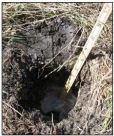
**Figure 5:** Measuring water level in a borehole.
