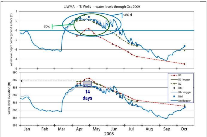
**Figure D3**: Water level monitoring data presented as depth below ground surface and as elevation. In the lower graph, water level elevation data are being used to determine the highest water level elevation attained for 14 consecutive days during a growing season.
