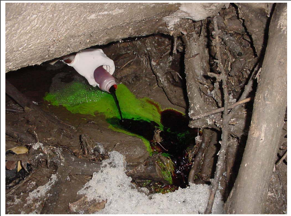
Figure 5. Introducing dye into the stream of water.
