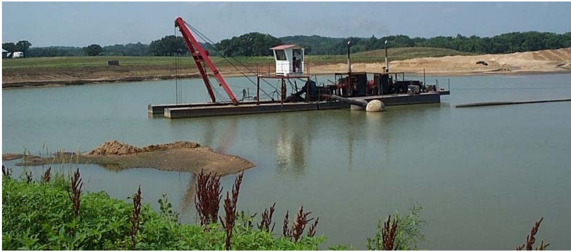
Figure 5. Donovan pit mining with a hydraulic dredge.
