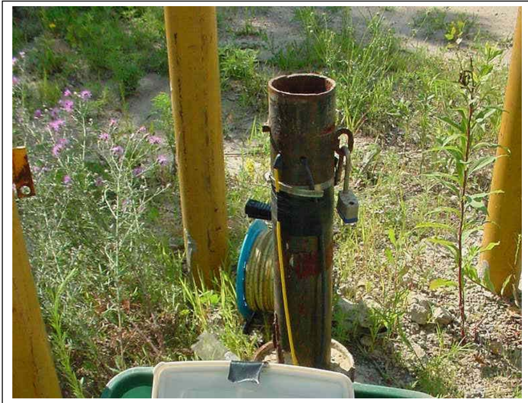
Figure 3. Water level measuring at a wellhead.
