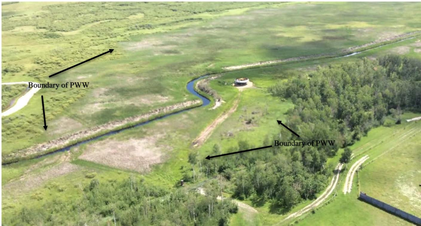
Figure 5. Image of the boundary of the public waters wetland along with the view of the overall impacts (ditch, UFO display/pad of fill). (Source DNR aerial video recorded on 8-1-19).
