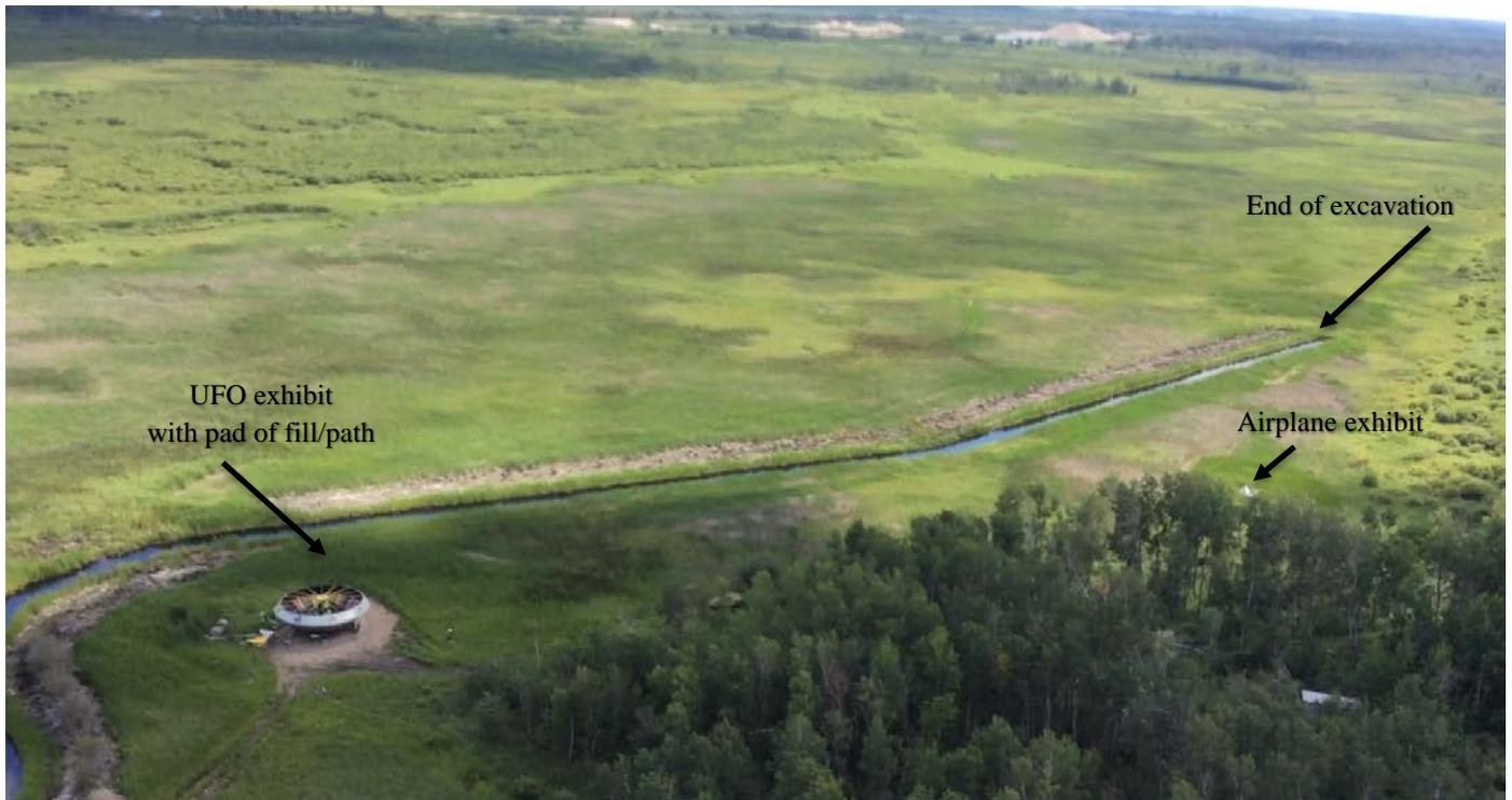
Figure 3. Image shows a closer view of the UFO and fill pad, the airplane exhibit and constructed ditch in the background terminating in the public waters wetland. (Source: DNR aerial video recorded on 8-1-19)
