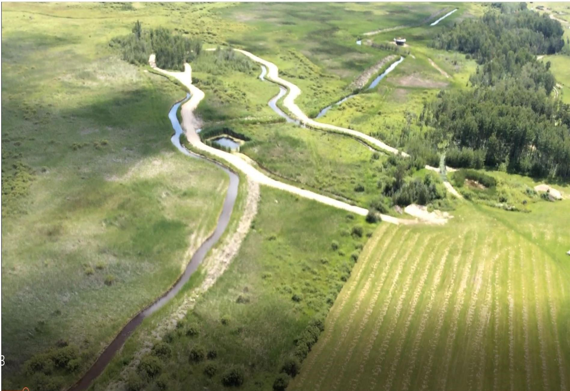
**Photo 3: Showing ditch with spoil extending past the new road. Also showing the gravel fill for the amusement ride.**
