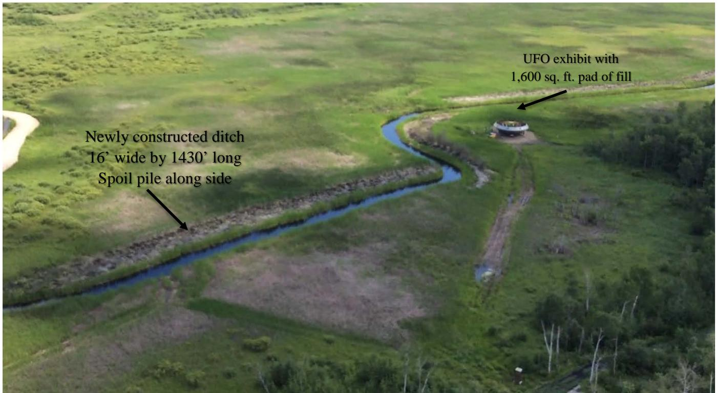
Figure 2: Image shows the constructed ditch and UFO display and pad of fill in wetlands (Source: DNR aerial video recorded on 8/1/19)
