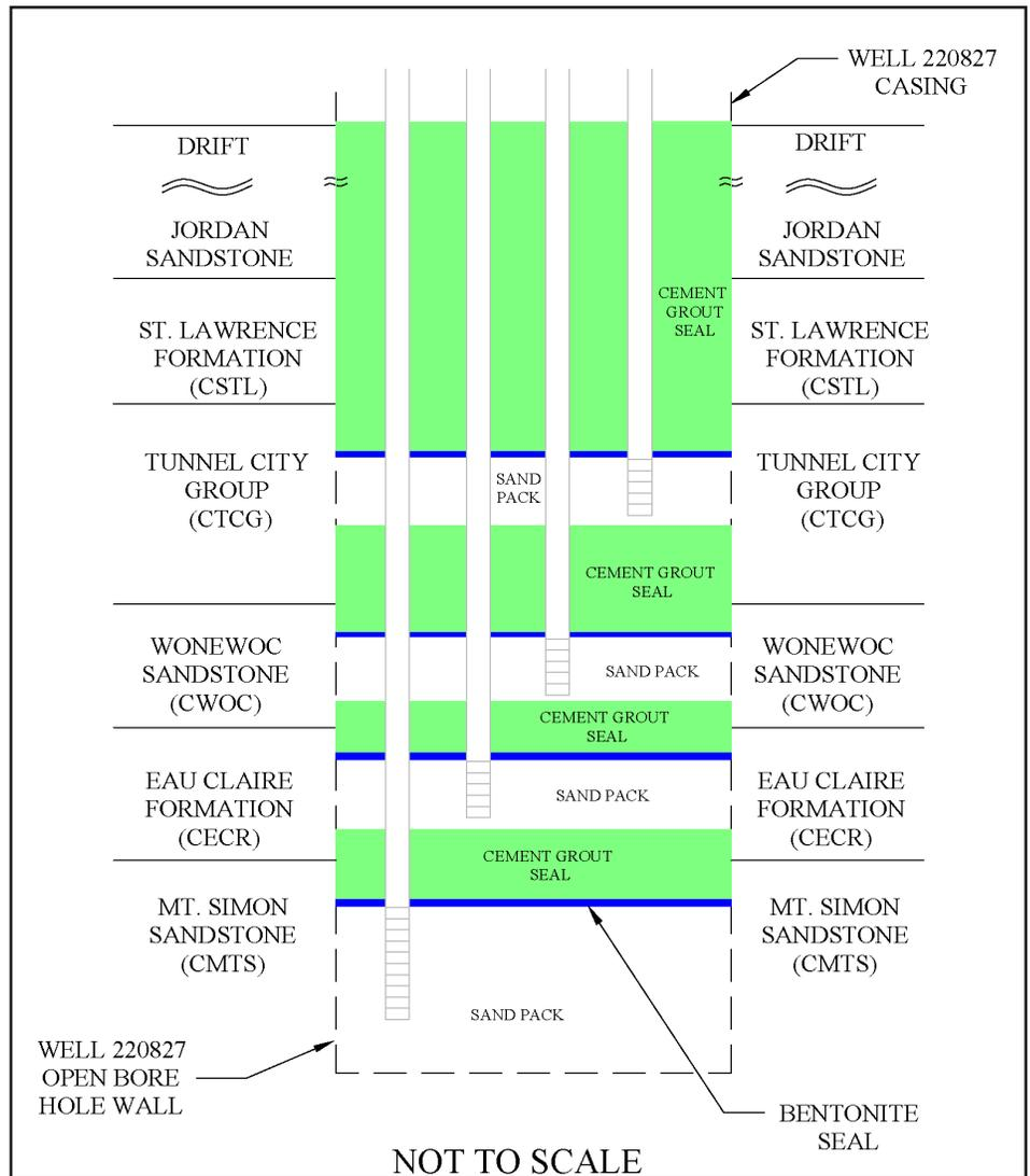
*This schematic diagram depicts four new monitoring wells (referred to collectively as a well nest) located on the site of the now-sealed RPU Well No. 16 in Rochester. The well nest will be used to collect data about water quality and water levels' stability in four aquifers.*
