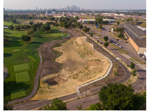
Previously untreated runoff from 612 acres now flows from east to west through Columbia Golf Course and Columbia Park, where it is diverted to a treatment pond, a dry basin, and then an infiltration basin before it re-enters the stormwater sewer system and continues on for 1.2 miles to the Mississippi River. The Clean Water Fund-supported project is slated to wrap up this month. Photo Credits: Mississippi WMO
