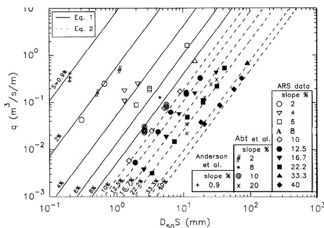
Figure 2-Rock chute stability data.
