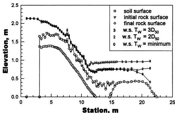
Figure 4-Bed and water surface profiles, 22.2% slope,  $D_{50} = 188$  mm, and  $q = 0.351$  m<sup>3</sup>/s/m.
