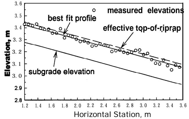
Figure 3-Top-of-riprap elevation.
