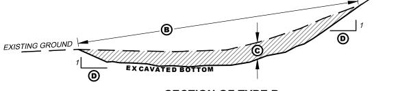
SECTION OF TYPE B SCRAPE / SEDIMENT REMOVAL
