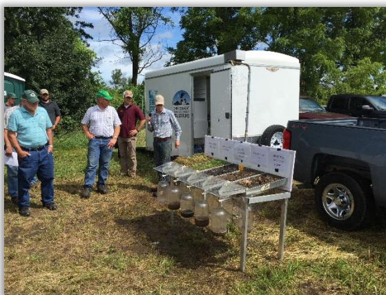
Rainfall simulator in use at the field day in Eyota.
