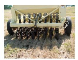
Equipment and materials for drill seeding include: Truax, Tye, Nesbit, Great Plains, and John Deere Rangeland seeders. Native seed drills have been constructed to accommodate different shapes and sizes of seed and use small plows or disks to open furrows. Seed drills also cover the seed with soil and pack with rubber rollers to ensure good seed-to-soil contact (Fuge 2000).
