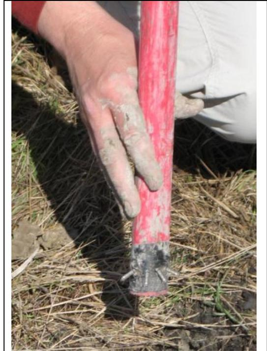
**Figure A9:** Homemade scarifying tool made with screws and plastic pipe.
