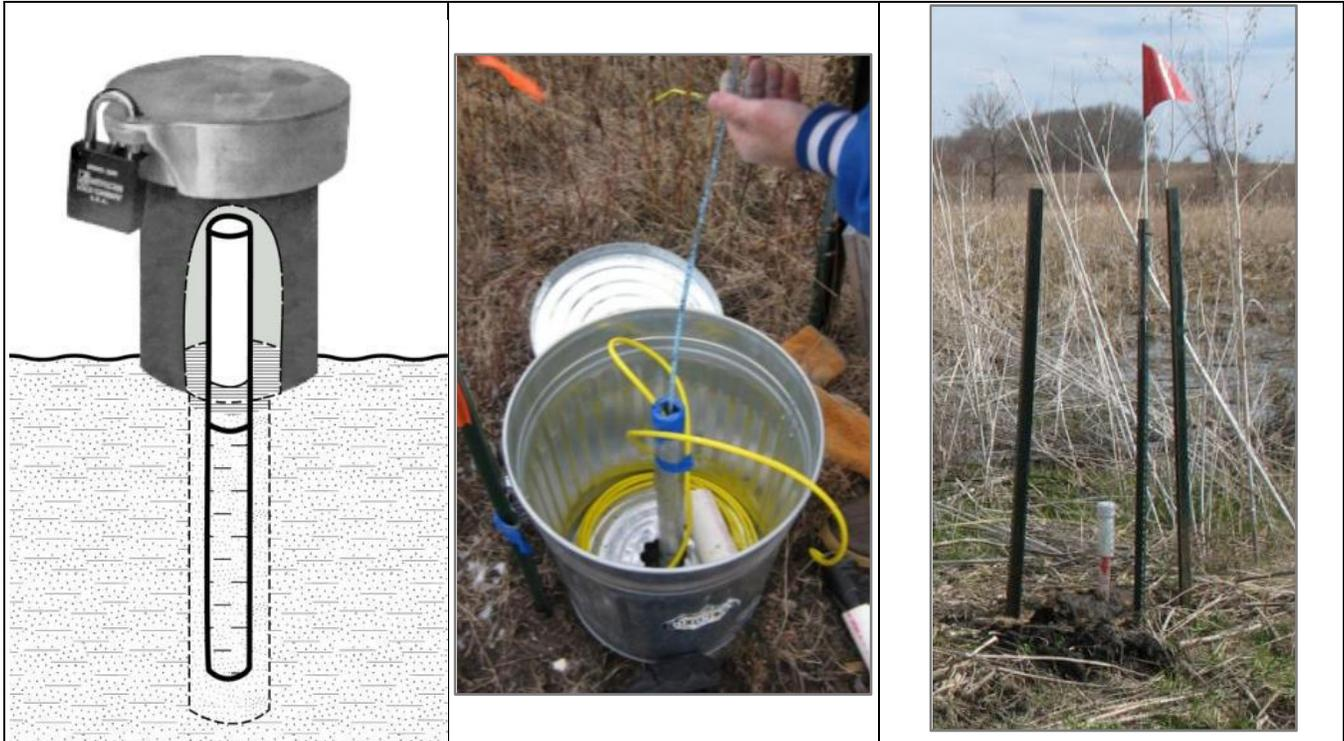
**Figure A5** Left: steel protective casing and locking cap. Center: Improvised protective housing for water level data logger. Right: Protection posts.
