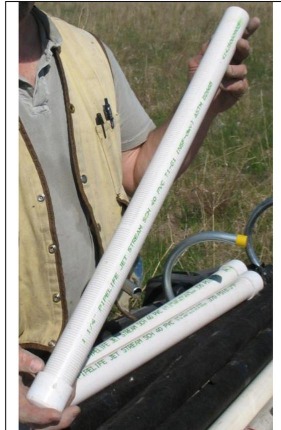
**Figure A2:** 1¼ - inch PVC monitoring well screen with bottom cap.
