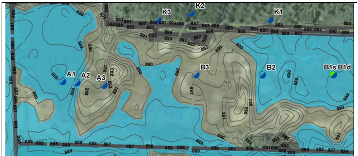
Figure D4: Map showing area where water table is within 12 inches for \geq 14 days during a growing season. Based on water level elevation data from monitoring wells and topographic survey.
