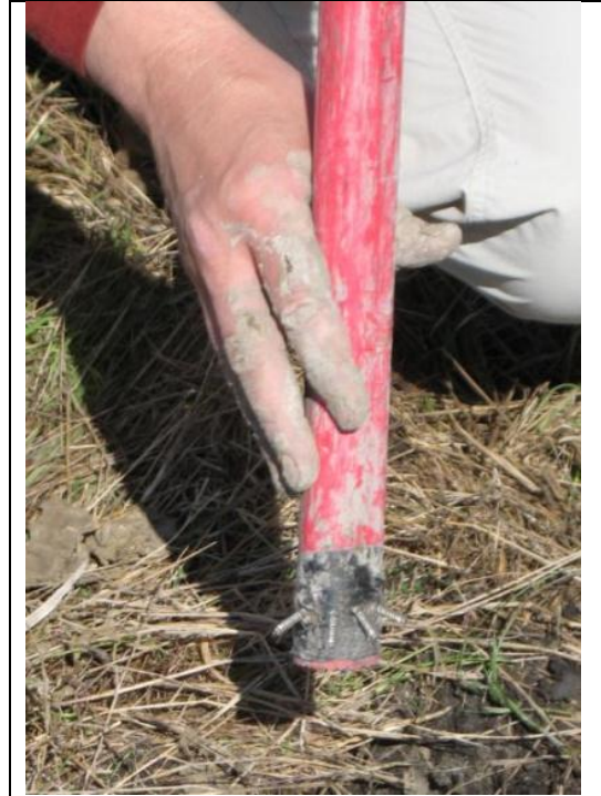
Figure A9: Homemade scarifying tool made with screws and plastic pipe.
