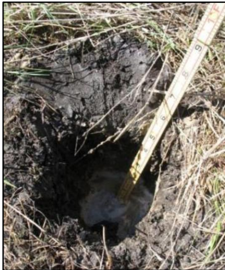
Figure 5: Measuring water level in a borehole.
