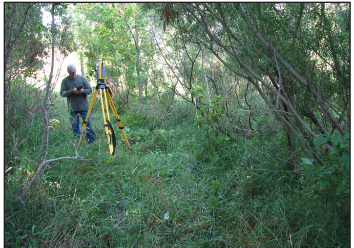
Right: An engineer uses total station equipment — a traditional system — to collect elevation data.
