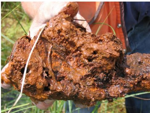
*Rust-colored particles drop out of the water emerging from the fen, often forming a rock-hard crust.*
