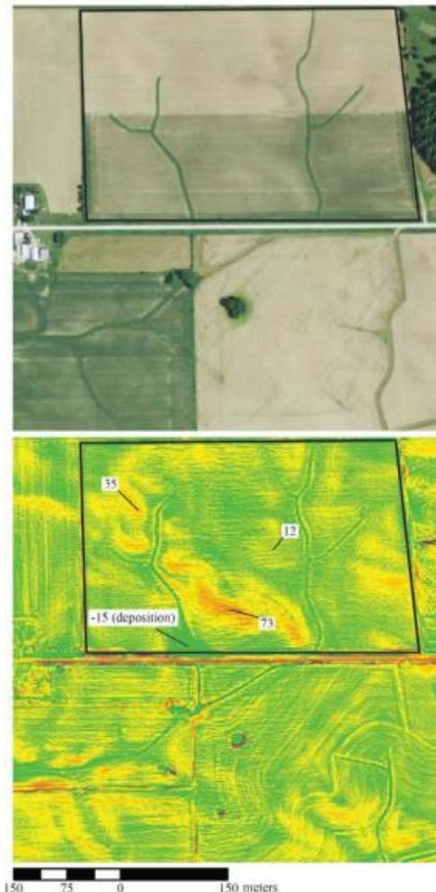
*For this field in Dodge County, the overall field average erosion rate is 2.7 tons per acre per year. Areas of potentially high soil erosion are marked in red.*
