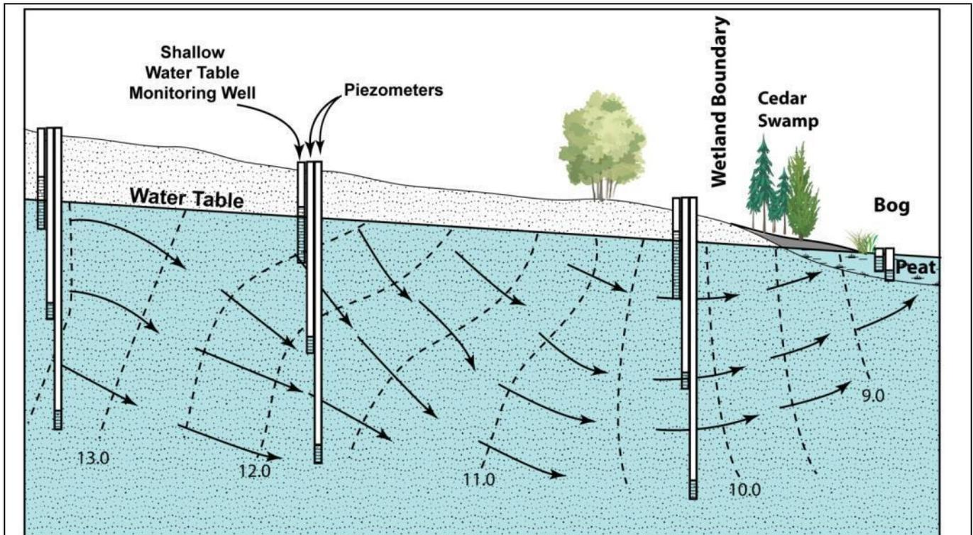
**Figure 18:** An example transect of shallow monitoring well/ piezometer “nests” as might be installed to investigate ground water flow at a wetland margin. The water levels measured in the piezometers give the hydrostatic pressure or “head” at specific depths. These can be used to construct a “flow net”. Contouring the head data yields lines of equal head (“equipotential” lines – dashed lines in figure), from which localized flow directions can be determined (arrows).
