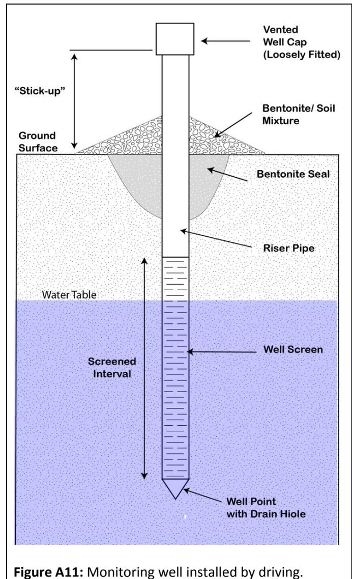
**Figure A11:** Monitoring well installed by driving.
