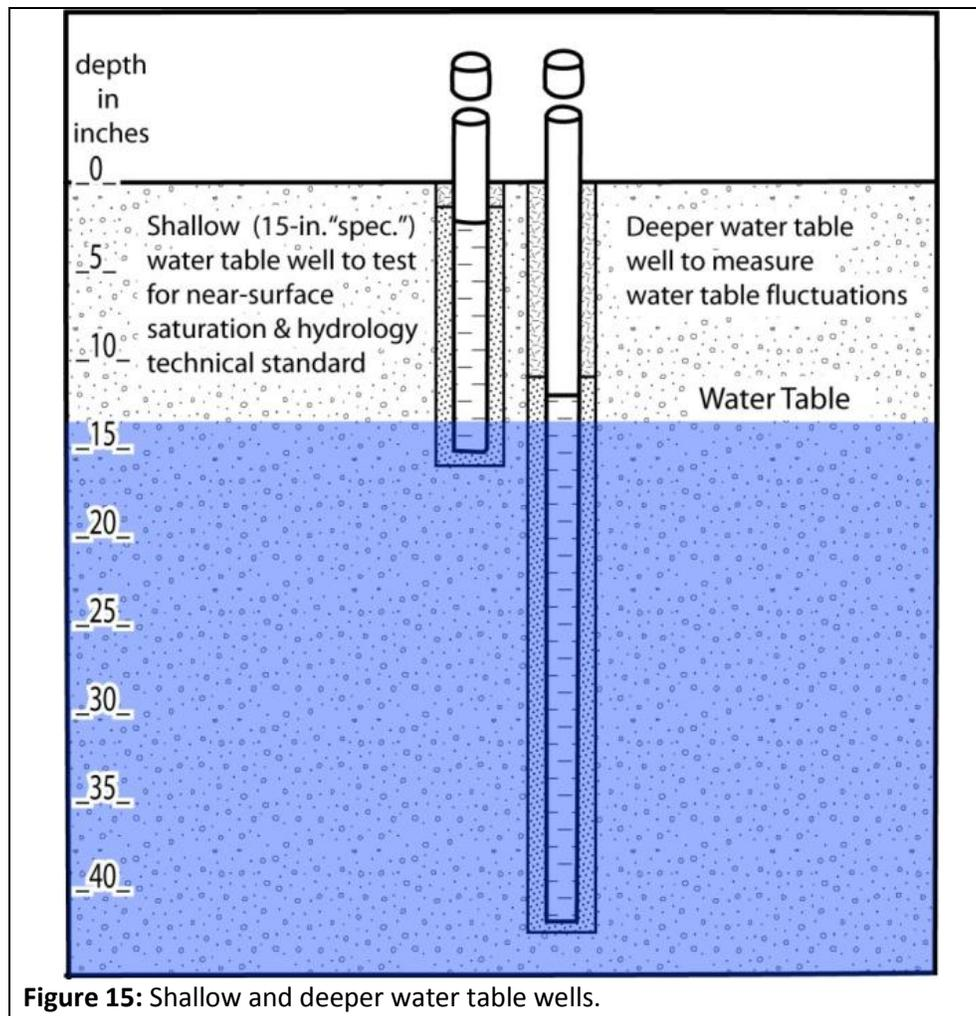
**Figure 15:** Shallow and deeper water table wells.
