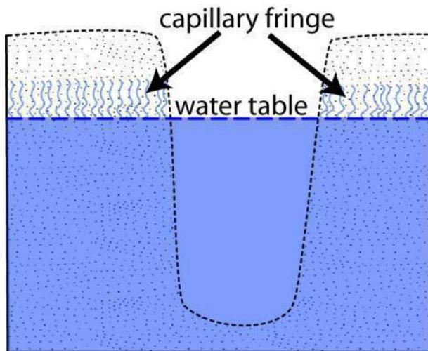
Figure 7: Water table and capillary fringe.
