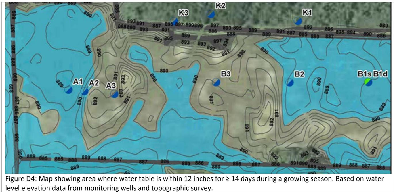
**Figure D4:** Map showing area where water table is within 12 inches for  $\geq 14$  days during a growing season. Based on water level elevation data from monitoring wells and topographic survey.
