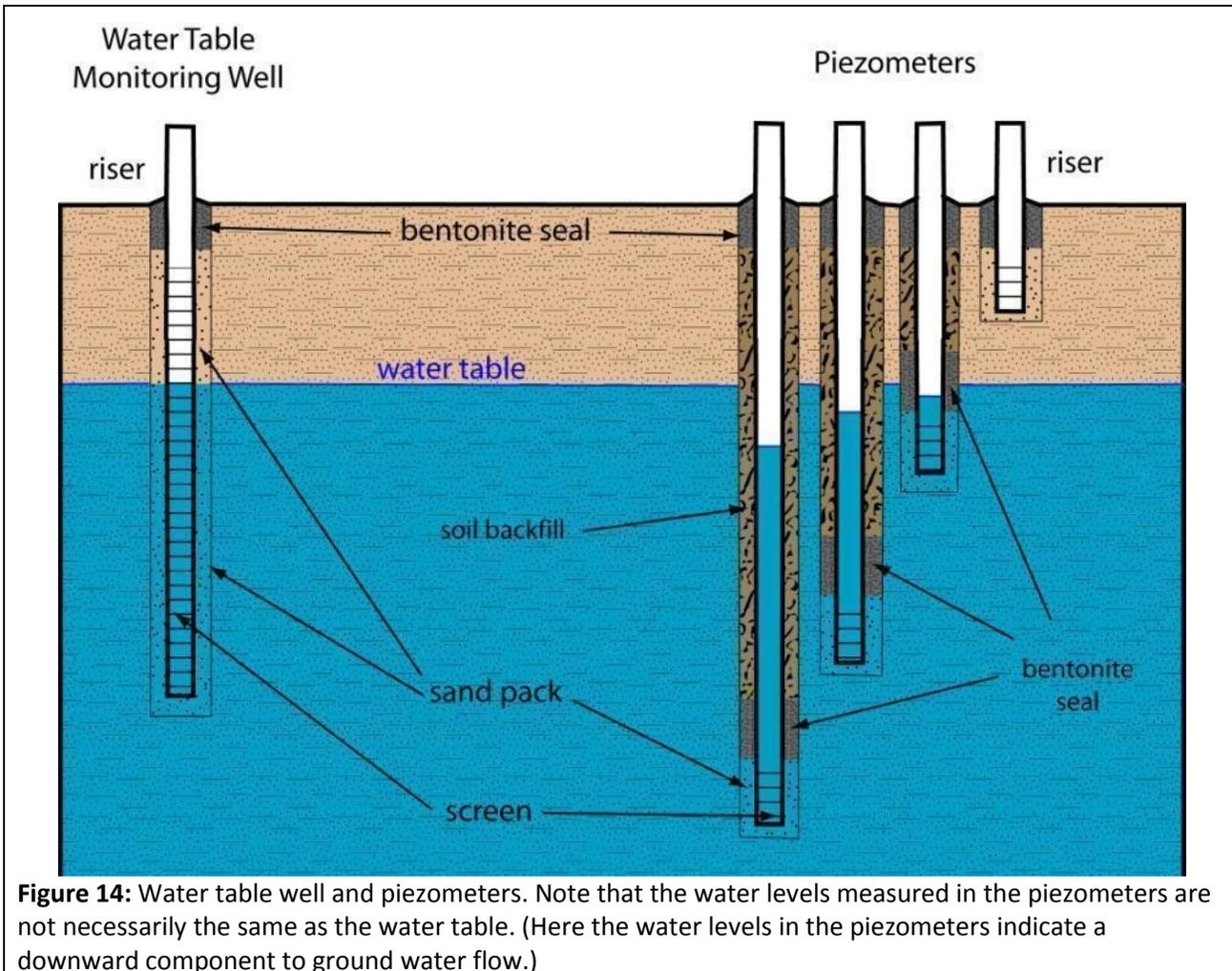
**Water-table monitoring wells** (also referred to as “**water-table wells**” or simply “**monitoring wells**”) are screened over a longer length – often from just below ground surface to the bottom of the pipe (**Figure 14** - left). They are designed to capture the water table within the screened interval. The water level inside a water-table monitoring well is the elevation of the surface of the groundwater rather than a pressure head at some point deeper than the water-table surface.
