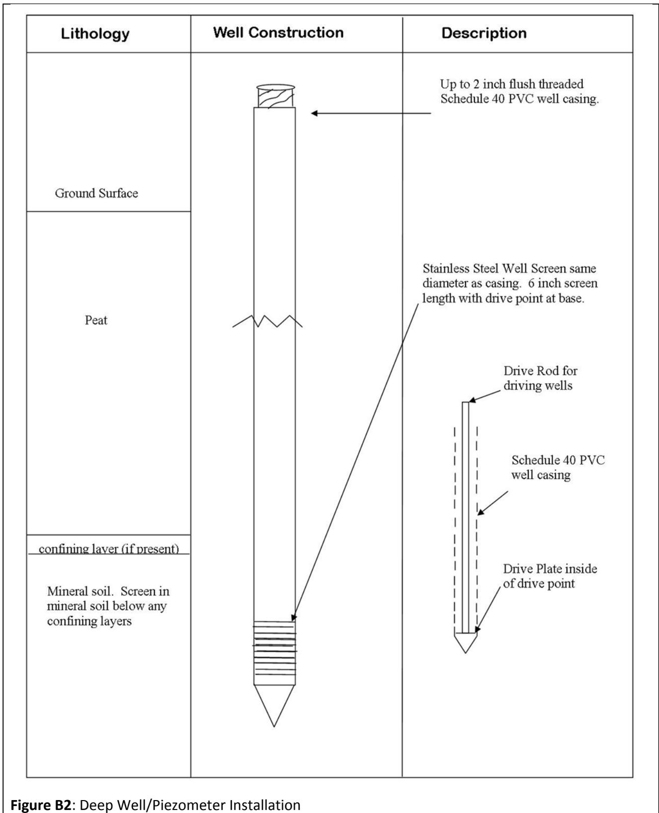
**Figure B2: Deep Well/Piezometer Installation**
