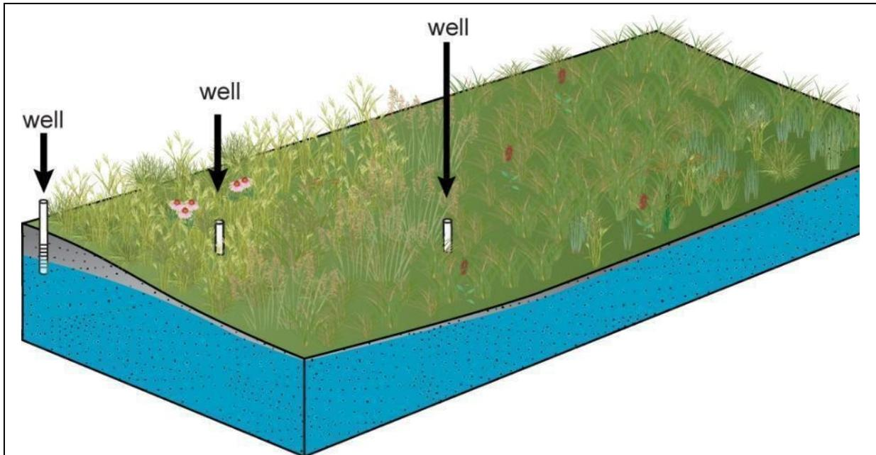
**Figure 16:** Monitoring using a transect of shallow wells.
