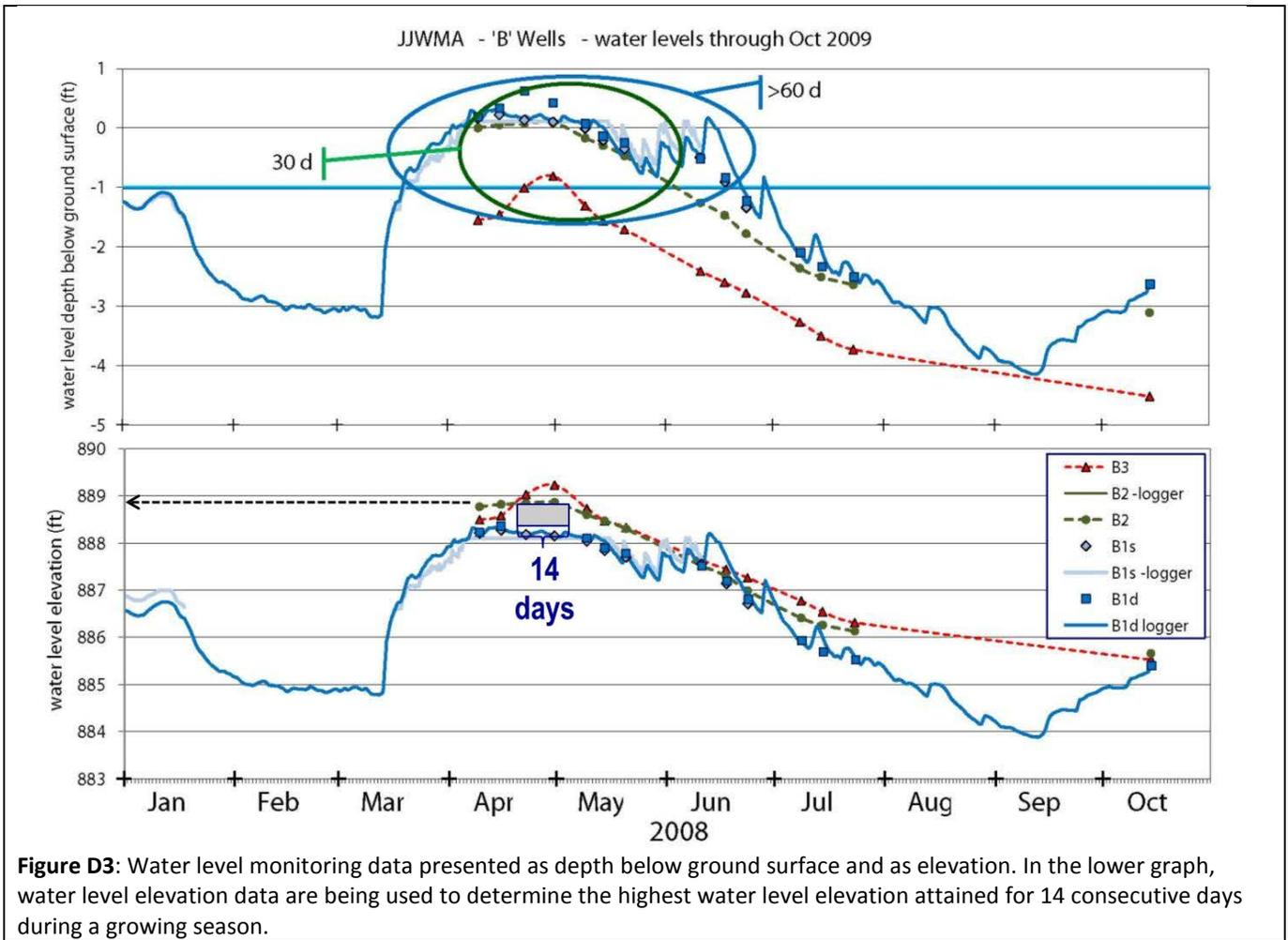
**Figure D3:** Water level monitoring data presented as depth below ground surface and as elevation. In the lower graph, water level elevation data are being used to determine the highest water level elevation attained for 14 consecutive days during a growing season.
