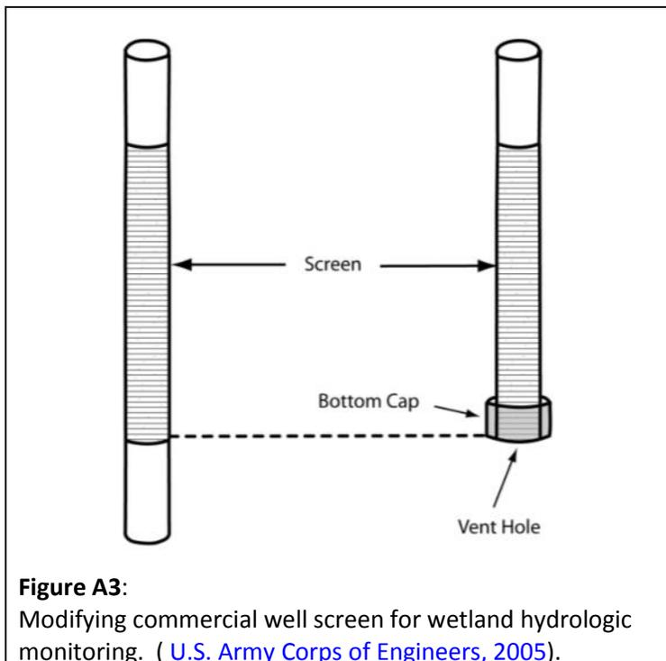
**Figure A3:** Modifying commercial well screen for wetland hydrologic monitoring. ([U.S. Army Corps of Engineers, 2005](#)).
