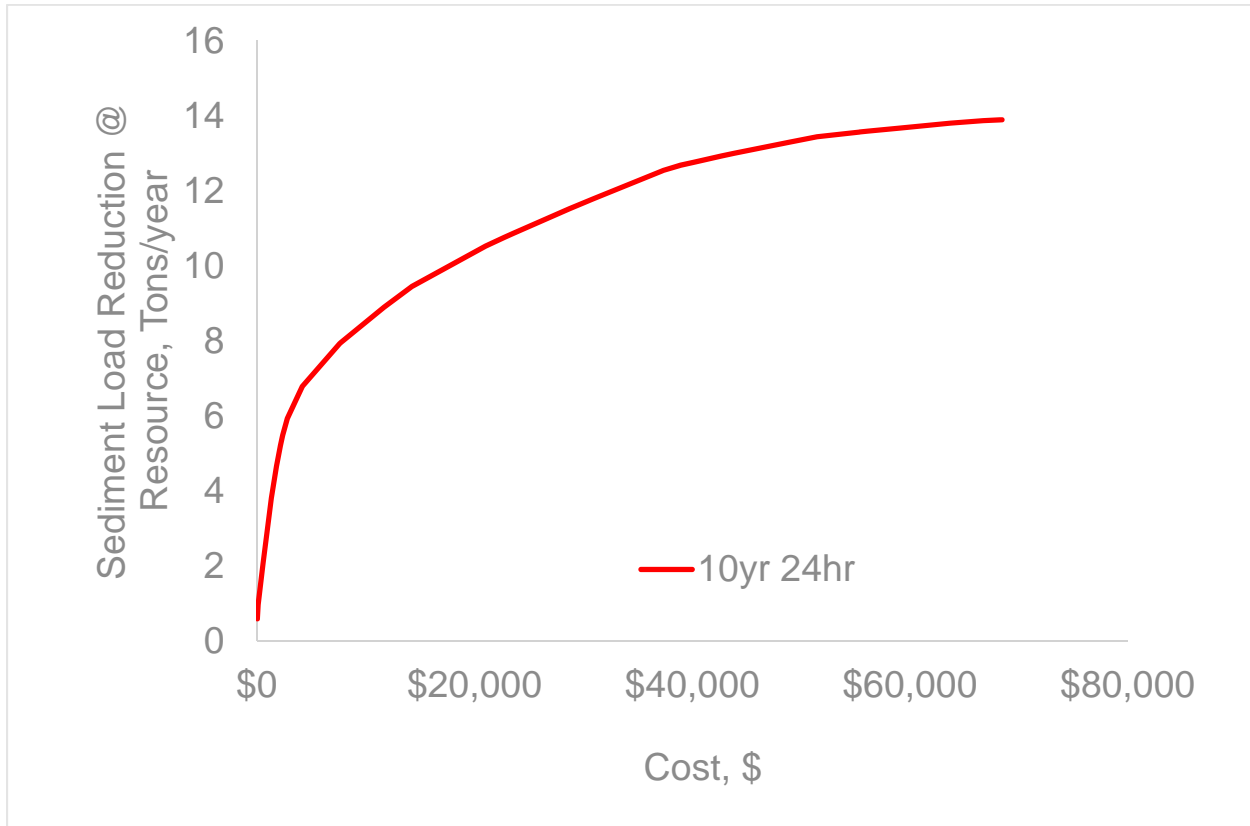
Figure 6. Single treatment efficiency frontier for filtration practices. Frontier indicates the maximum reduction in sediment delivered to the main channel of the Sand Hill River relative to the implementation cost.
