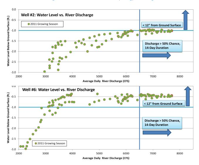
Figure 14: Graphs of water levels in wells #2 and #6 vs. average daily river discharge, now with the added 50% probability 14-day duration river discharge of **6560 cfs** (vertical line).
