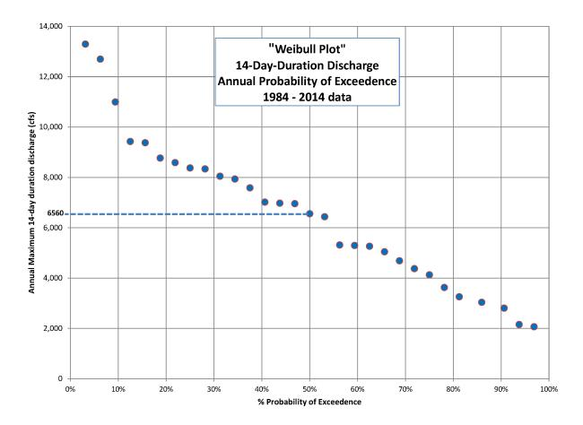
**Figure 15:** Plot of the annual probability of exceedance of 14-day-duration discharges (Weibull Plot"), based on 1984-2014 data. It shows the probabilities that a discharge will be met or exceeded for 14 days in a year. The number we are interested in is the **50% annual probability** – i.e. the discharge that will be reached or exceeded for 14 consecutive days in **most years**.
