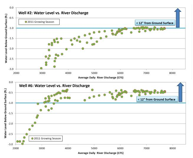
Figure 10: Graphs of water levels in wells #2 and #6 vs. average daily river discharge in cubic feet per second (cfs).
