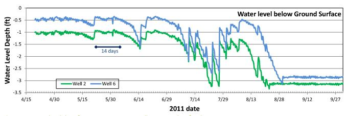
Figure 7: Water-level data from two monitoring wells in Example 2 for the 2011 growing season.
