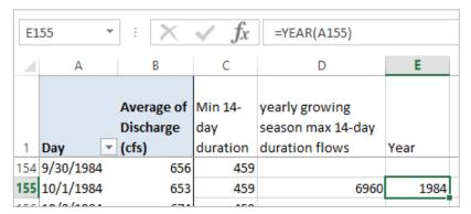
**Figure 12:** The formula =YEAR(A155) in Column E calculates the year from the date in Column A. This is useful for sorting the maximum values into a new column.
