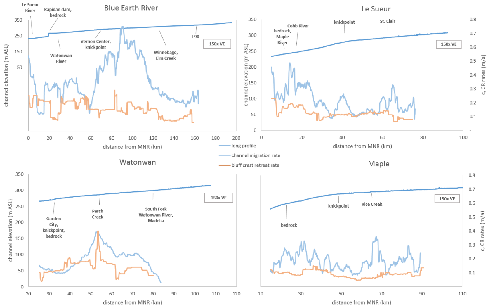
Figure 5.5: Bluff crest retreat and channel migration rates, smoothed over a 3 km radius. Channel migration rates include bluffs, banks and bedrock reaches, but not reaches that avulsed or were shortened from 1938 to 2008. Long profiles have 150x vertical exaggeration. Figure from Bevis (2015).
