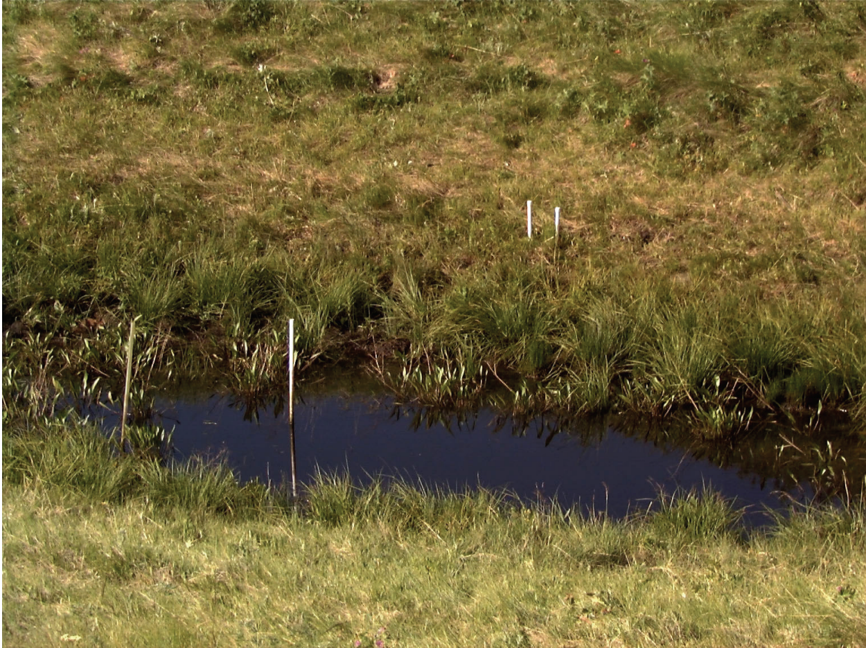
Figure 7. Water table monitoring wells near the center and edge of a depressional wetland
